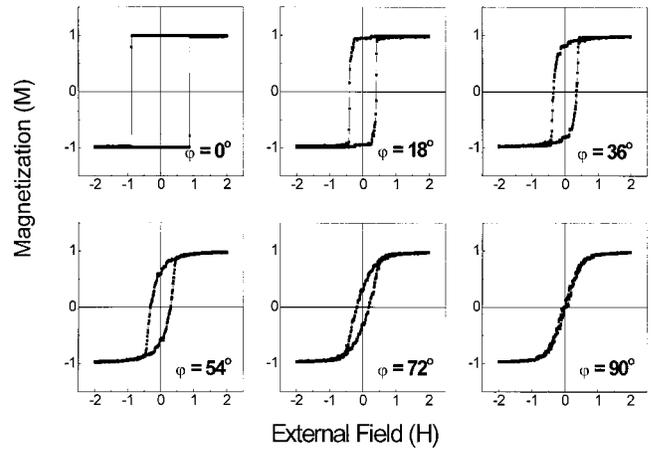
FIG. 2. Simulated hysteresis loops for  $t=4$  and  $s=1/5$ , at different angles,  $\phi$ , between the direction of the external field and the step direction:  $\phi=0^\circ, 18^\circ, 36^\circ, 54^\circ, 72^\circ$ , and  $90^\circ$ .
