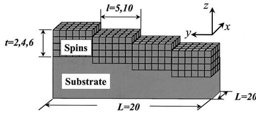
FIG. 1. Schematic diagram of simulation samples. The sample size is chosen to be  $20 \times 20 \times t$ , where  $t$  is the thickness of the film chosen to be two, four, and six atomic layers ( $t=2, 4$ , and  $6$ , each with two step densities  $s=1/5$  and  $1/10$ ). Periodic boundary conditions are used in the plane of the film surface and free boundary conditions are used in the direction normal to surface. The interaction between the substrate and the magnetic film is ignored.
